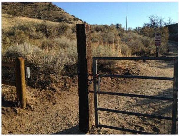
Portable bicycle and pedestrian counting equipment, like this one in the Boise foothills, measures direction of travel and general counts using an infrared sensor.
