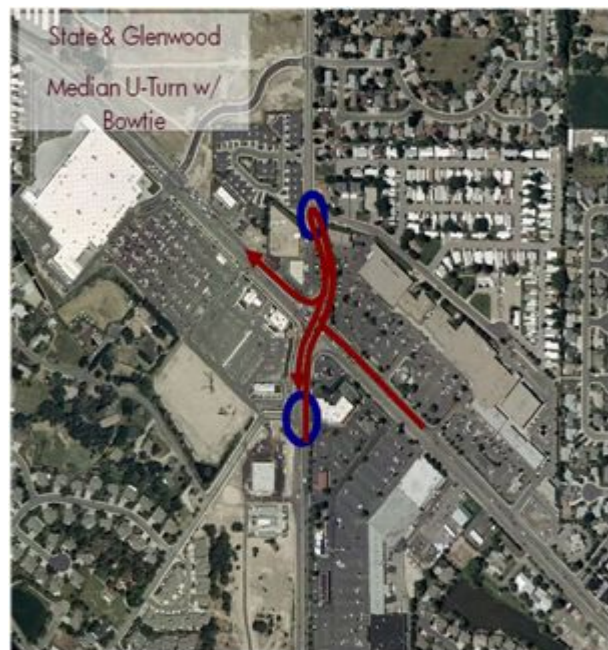
Figure 2-11: Median U-Turn with Bowtie
