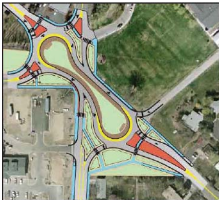
Figure 7-7: 36 th Street/Hill/Catalpa Preliminary Design
