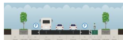
ACHD's concept for Fairview Avenue on the west end calls for one less traffic lane, street parking on both side and a protected bike lane. Image courtesy of Ada County Highway District.
